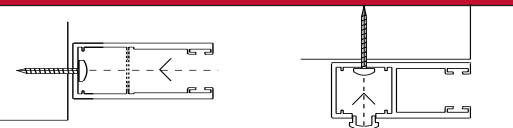
Detail: Guide reveal fixing Detail: Guide Face fixing
